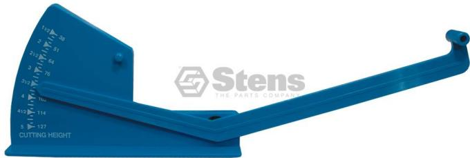
**Leveling Gauge Plastic** Used to accurately level and measure mower decks on all riding and walk behind mowers. Mower blade cutting height gauge range is 1 1/2" to 5". Measure tip to tip cutting edge (side to side and front to back).- Measure one side cutting edge. Check height on gauge.- Measure other side cutting edge. Check height on gauge.- Deck is level if heights are the same. If not, deck adjustments will need to be made. **USE GLOVES TO AVOID INJURY**
